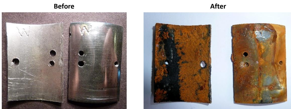
When water comes into contact with ethanol blended petrol it draws the ethanol out of the petrol making the water acidic. It is this acid that attacks the metal components. This problem is as serious with current petrol blends as it will be with E10. All it needs is a single drop of rainwater getting into the fuel system.
